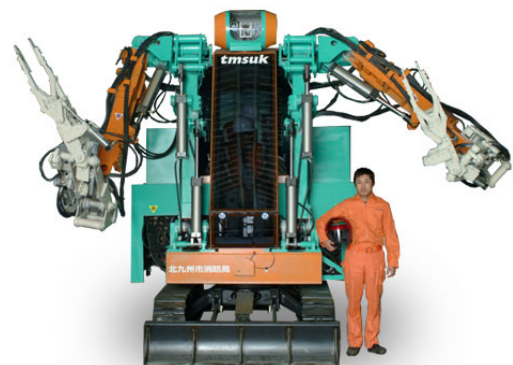
Illustration 2: T-52 Enryu Rescue Exoskeleton A 5 ton 10 foot high hydraulic exoskeletal mechanism for cutting through debris after a disaster such as an earthquake.
