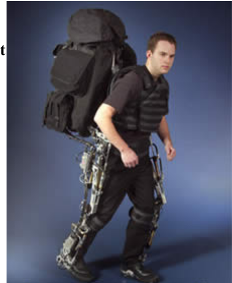
Illustration 1: The Berkeley lower extremity exoskeleton can be used to augment soldiers' ability to carry heavy equipment for long periods of time.
